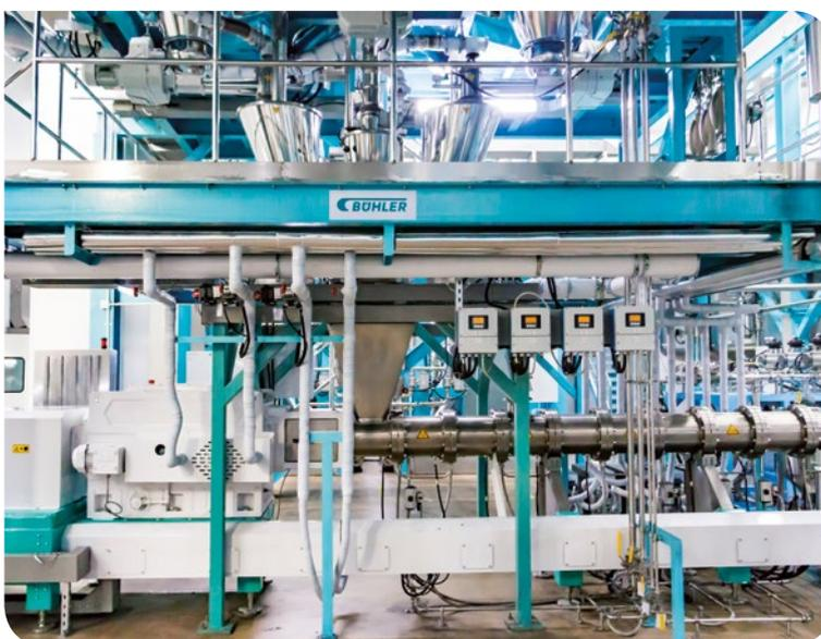
Lithium-ion batteries from the Chinese manufacturer Lishen can be found in all sorts of devices, from smartphones to wearables and notebooks. The next major field of application for Lishen is energy storage systems for electric vehicles. The company has been joined on this venture by the Bühler Group to redefine the manufacture of electrode paste by introducing a new process.
